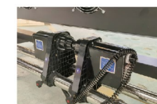
External power supply, intelligent rolling system
