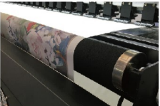
Front expander ensure quick and accurate take-up in high speed printing.
