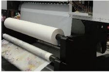
Rear loading and take-up to facilitate workflow.
