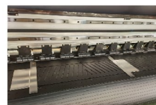
Honeycomb suction platform ensure the flatness of the paper more effectively when printing .
