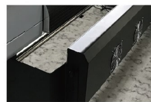
Infrared heater and cooling fan.
